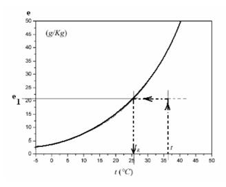
fig.2 Specific humidity vs. temperature
